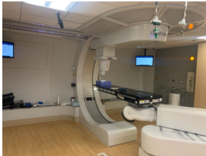
Figure 3. Mevion S250 proton radiation therapy system at Orlando Health. Seeds were placed in the beam path on top of the blue solid water block.
