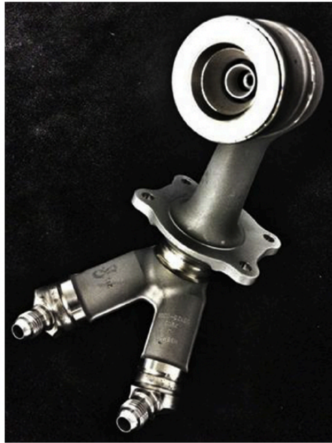
Fig 7: GE leap engine fuel nozzle created using direct metal laser melting via the EOS metal powder bed fusion machine [Liu et al. 357].
