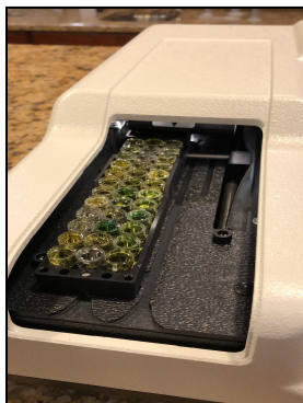
Figure 3: ELISA microplate reader with test samples
