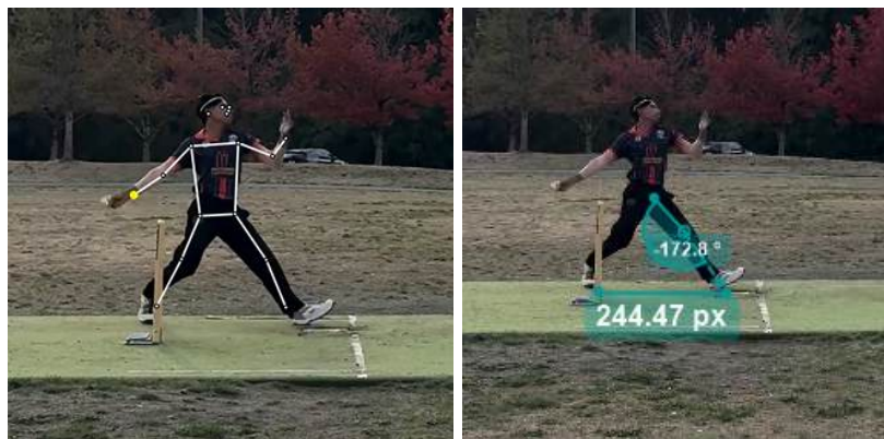
Figure 7: Subinay Kalya's estimated Knee Angle @FFC was 174.7. The manual Calculation shows 172.8, a difference of only 1.9 degrees. His Stride Length was estimated at 1.15m; converting 244.47px to meters yielded 1.23m.
